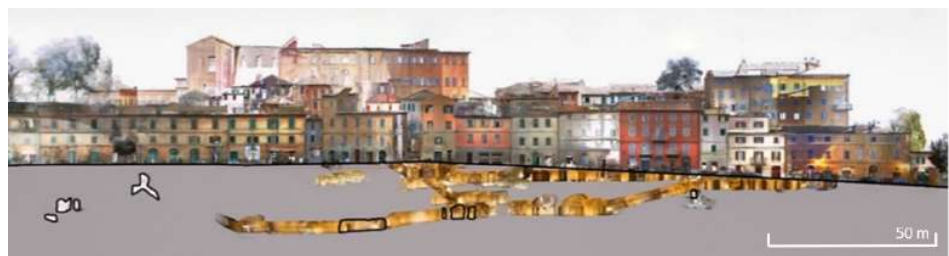
Figure 2. Vertical section of the city center of Camerano (Italy) with the underground caves.
