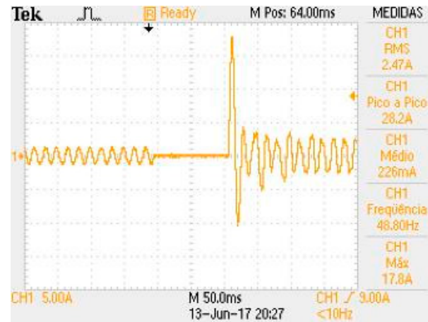
Figure 5. Typical current waveform for the common form of delta connection— \Delta t = 100 ms. (Vertical scale—5 A/division; Horizontal scale—50 ms per division).
