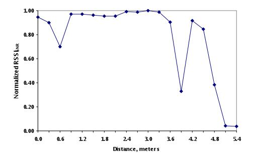
Figure 6. RSSI<sub>SNR</sub> dependence on distance (Nokia).
