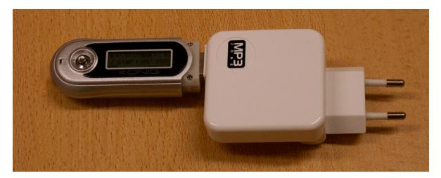
Figure 2. MP3 player with an embedded FM transmitter, connected to power adapter. (The antenna is not attached.)
