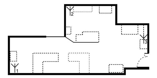
Figure 1. Floorplan of the measurement area. The antennas mark the positions of the three transmitters and the dashed lines mark room furniture.
