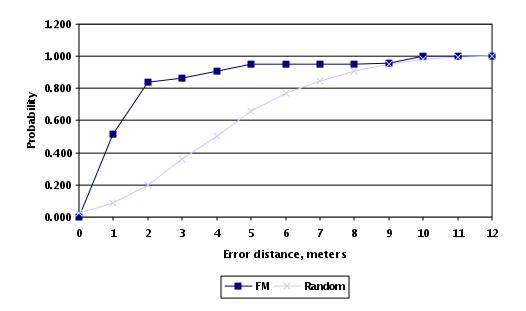
Figure 7. Error distributions for two-dimensional positioning (HTC).
