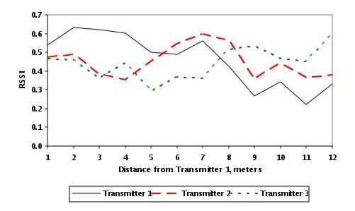
Figure 5. RSSI variation while moving from Transmitter 1 to Transmitter 3, with Transmitter 2 placed between them (Nokia).
