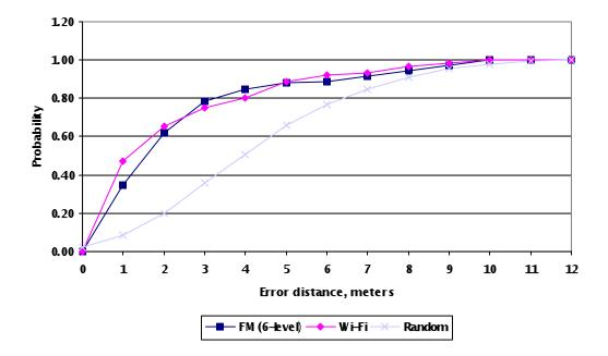
Figure 8. Comparison of Wi-Fi and FM error distributions (HTC).
