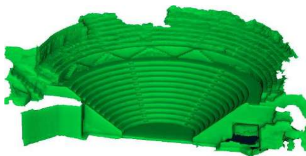
Figure 9: Polygonal model generated with Poisson algorithm.
