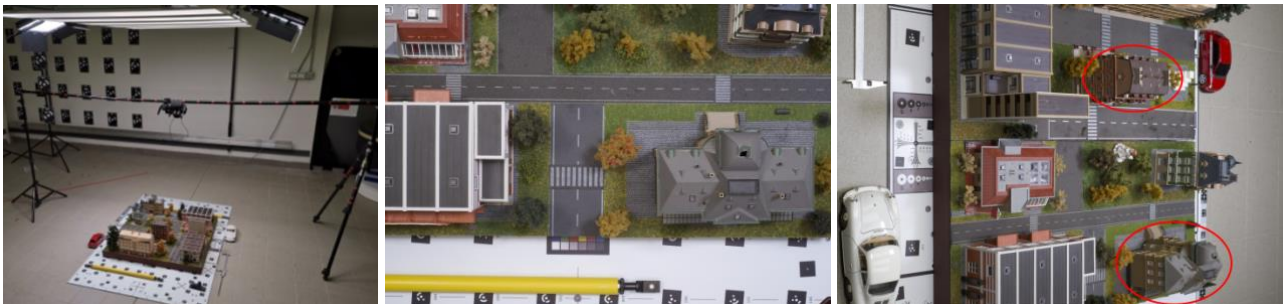
Figure 1. The test-object and acquisition scenario adopted for the 3DOMcity photogrammetric contest: setup for data collection (left) and examples of nadir (centre) and oblique (right) images. Red ellipses highlight the buildings selected for DIM evaluation.
