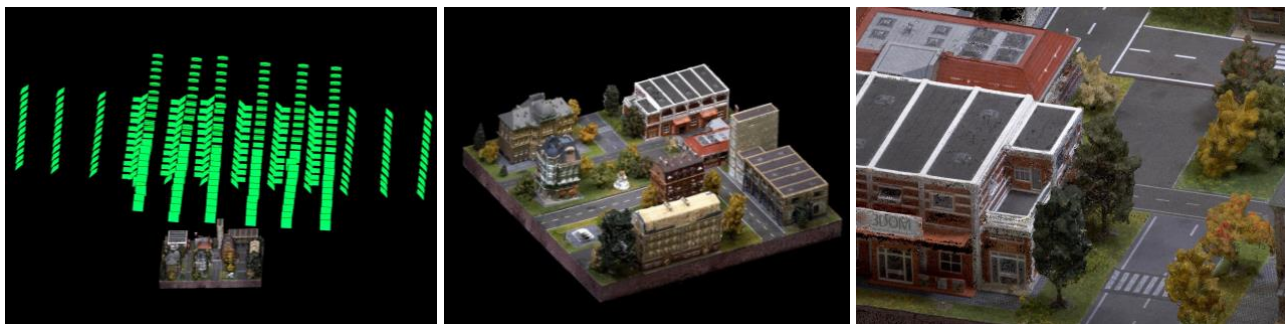
Figure 3. Examples of the datasets available within the “ 3DOMcity ” photogrammetric contest: reference image network (left), reference DIM point cloud (overview in center and close-up view on the right).
