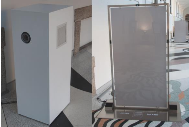
Figure 2 The structures of the Leonardo Plays Leonardo installation: on the left, the back-end wooden box; on the right, the stainless-steel frame with screen.
