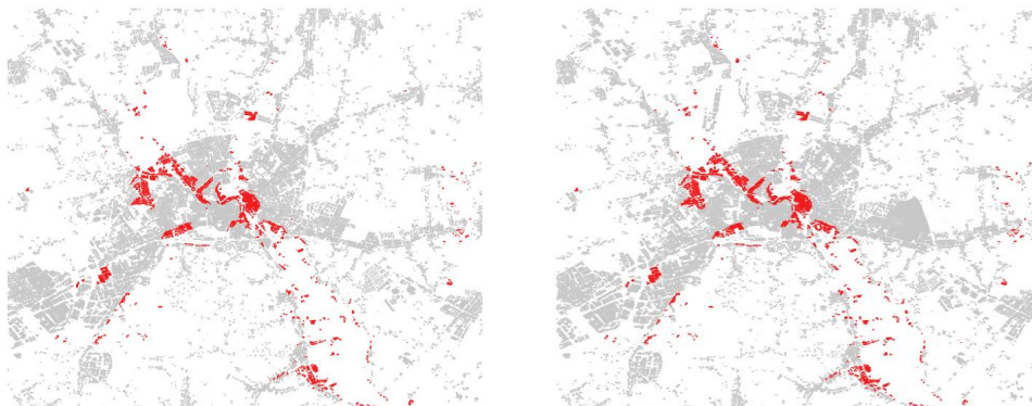
Figure 5: InaSAFE output layer no. 2: flooded building in Vicenza using official (L) and OSM data (R)
