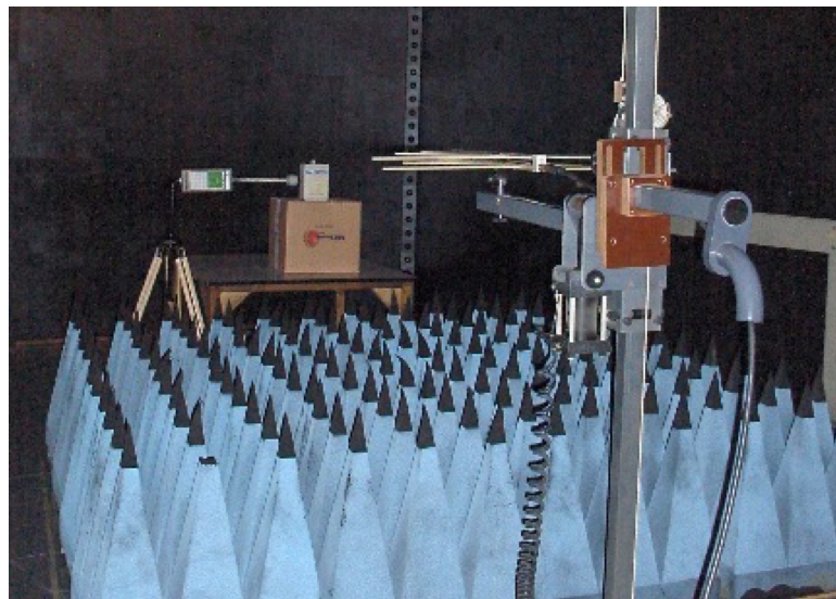
Figure 5. Experimental setup arranged into a semi-anechoic chamber. To obtain a circular polarization from a linear polarized antenna a circular polarization converter metasurface has been considered [18].
