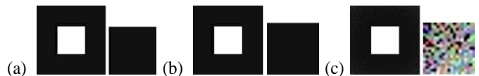
Fig. 8. (a, left) A toy image displaying a bright square over a dark one, and its color lightnesses by (b, left) STAR and (c, left) RSR ( N = 20, m = 100 ). The small squares in (a, b, c, right) are enlargements of the bottom right corner of the images on left. Enlargements have been equalized to allow the visualization of the noise generated by RSR. This noise is totally absent in the image processed by STAR.
