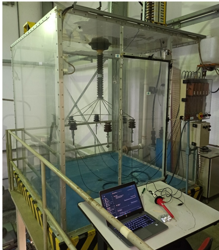
Figure 1. Salt fog chamber (high-voltage laboratory).
