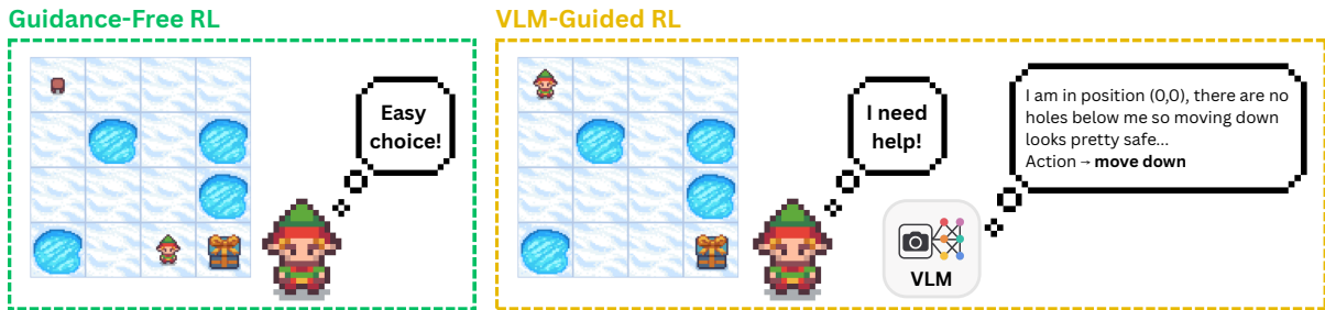
Figure 1: Dual architecture for RL: the agent is free to act in situations where it displays high confidence, but requests guidance from a VLM when it is uncertain, following the suggested action.
