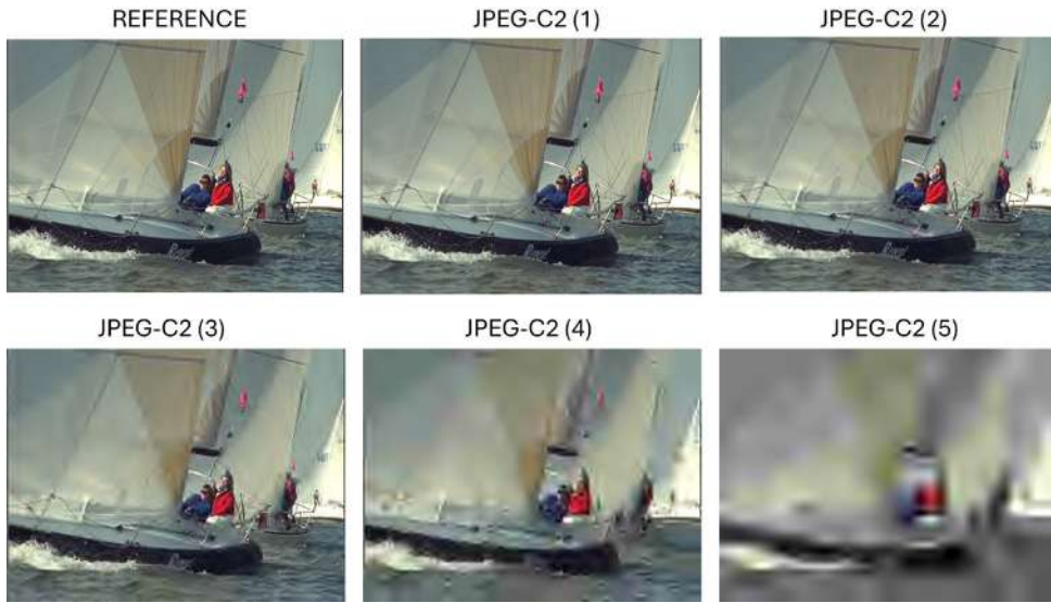
FIGURE 36. An example of JPEG2000 compressed image from TID-2013. The reference image undergoes to 5 different levels of compression indicated by JPEG-C2000(X) with X = 1, 2, 3, 4, 5.
