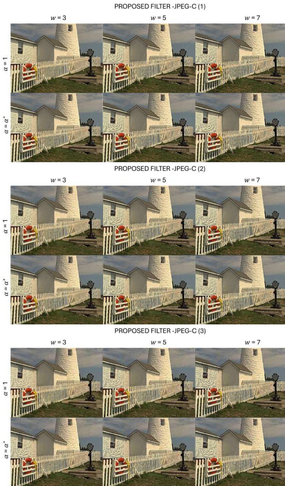
FIGURE 31. The results of the proposed sharpening algorithm on the first three JPEG compressed images in Figure 29. No edge over-enhancement is visible.
