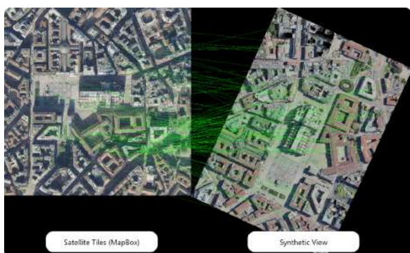
Figure 3. Example of image-matching between a satellite imagery tile (right) and a synthetic model view (left).
