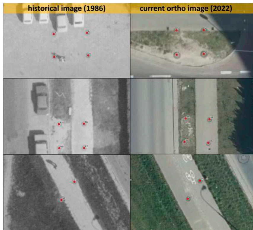
Figure 5. Examples of stable-over-time points measured in the field: points identified in the historical dataset (left panel) and the corresponding points in the modern orthophoto (right panel).
