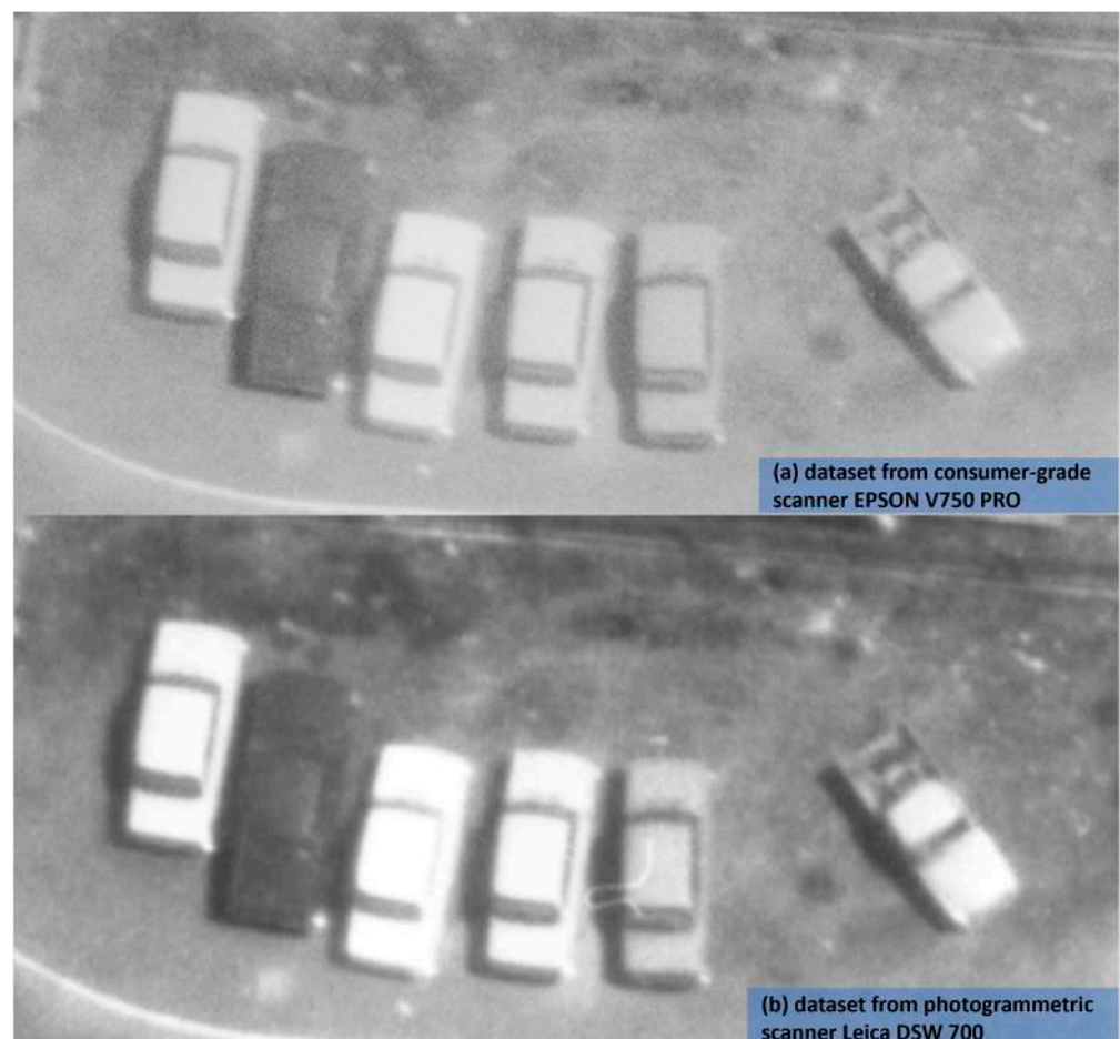
Figure 1. A view comparing the same image detail from a historical aerial picture scanned with the consumer-grade scanner EPSON V750 PRO (a) and with the photogrammetric scanner Leica DSW 700 (b).
