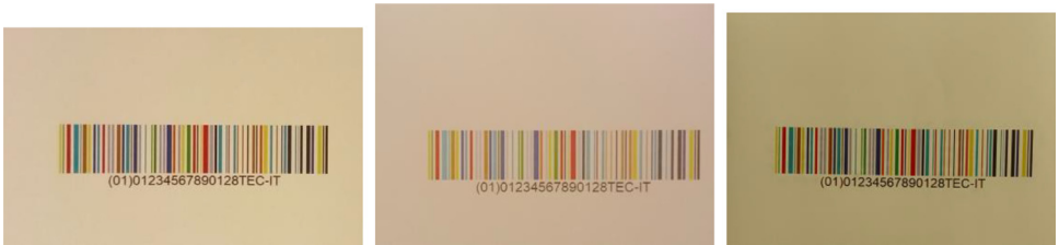
Fig. 3. Two images of a colour barcode, both acquired by Camera 1, printed on paper with density 80 gr/m 2 (on left) and 160 gr/m 2 (middle). On right, the image of the same barcode printed on paper with density 80 gr/m 2 but acquired by Camera 6. All these three images have been captured under the illumination Artificial-01. The colours of the left image appear different from those of the middle image because of the different kind of paper, printer, and ink as well as because of the automatic white balance performed by the used camera. The colours of the left image also differ from those of the right image because different cameras render colours differently.
