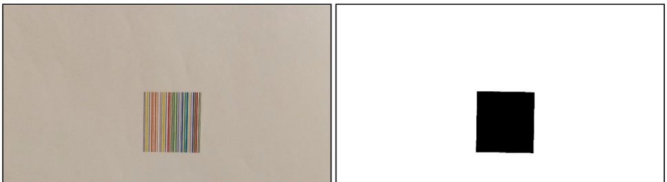
Fig. 4. On Left: An image with a colour barcode printed on paper with 80 gr/m 2 and acquired by Camera 1 under illuminant Artificial-01. On right: The mask of the image on left, i.e., the binary image whose black pixels specify the position of the colour barcode in the image. This mask has been computed by a semi-supervised segmentation algorithm, whose results were eventually refined manually – if needed. A black border has been added to the images to better show the mask content.
