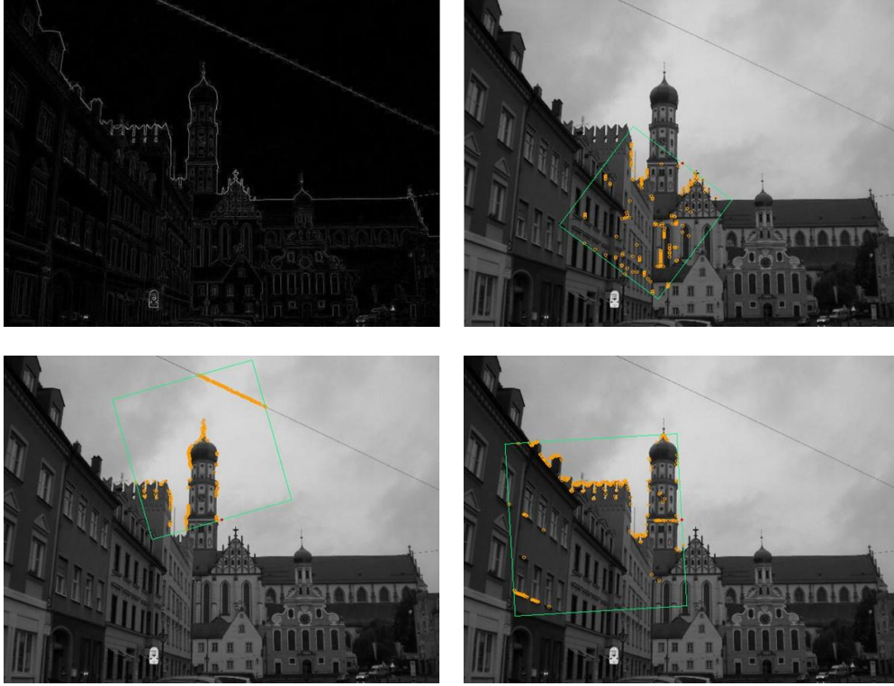
Fig. 3. The first image shows the gradient magnitude of the image in Figure 1. The other pictures show some random squares (in green) used to scan the neighborhood of the barycenter x of the image support (see Figure 1). These pixels maximize a function which is directly proportional to the gradient magnitude, while inversely proportional to their Euclidean distance from x .
