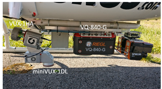
Fig. 2. Photograph of the scanner arrangement of the HeliALS system, showing the VUX-1HA scanner at \lambda = 1550 nm, miniVUX-1DL scanner at \lambda = 905 nm, and VQ-840-G scanner at \lambda = 532 nm.
