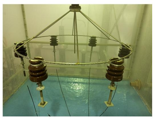
Figure 1. Insulators in a saline chamber experiment.
