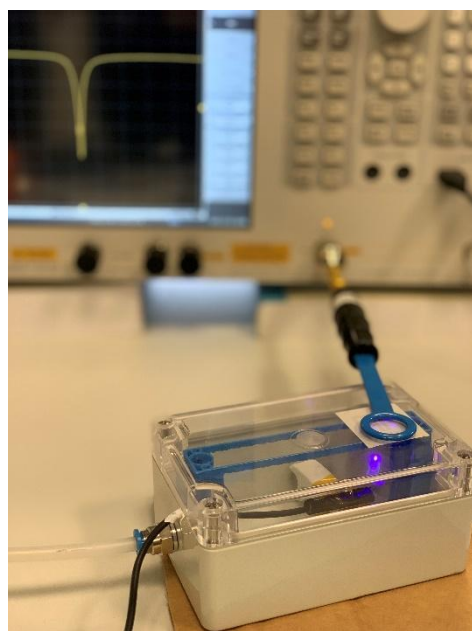
Figure 3. Picture of the custom-made gas chamber. The sensing probe is located outside the chamber, and the sensor is placed face-down to maximize the interaction with the chamber environment. The purple light is the UV LED source.
