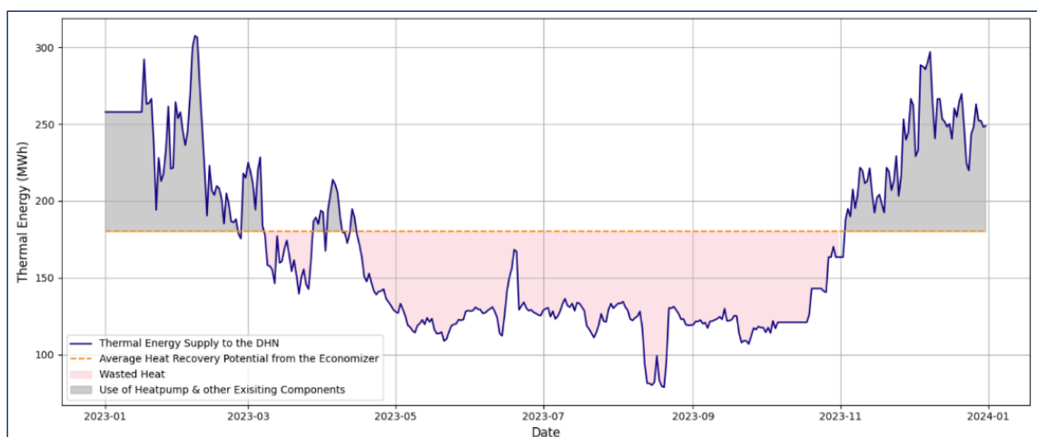
Figure 4. Daily thermal energy supply profile for district heating network (dark blue line) for Riva del Garda in 2023, highlighting the economizer recovery potential (orange dashed line), available excess heat during the summertime (pink area), and the utilization of other components to meet the peak demand during wintertime (gray area).
