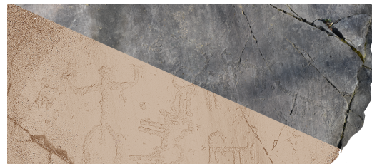
Figure 3: Example of photogrammetric dense point cloud, with/without color information.
