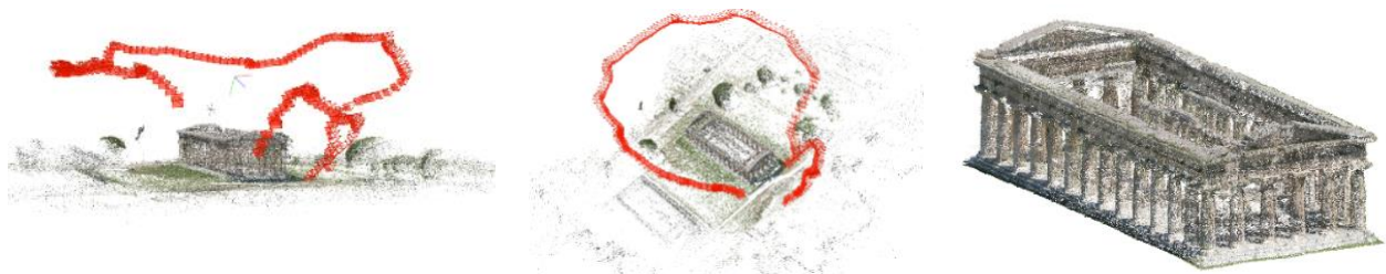
Figure 1. From UAV image network and sparse point cloud (left and middle) to dense point cloud (right).
