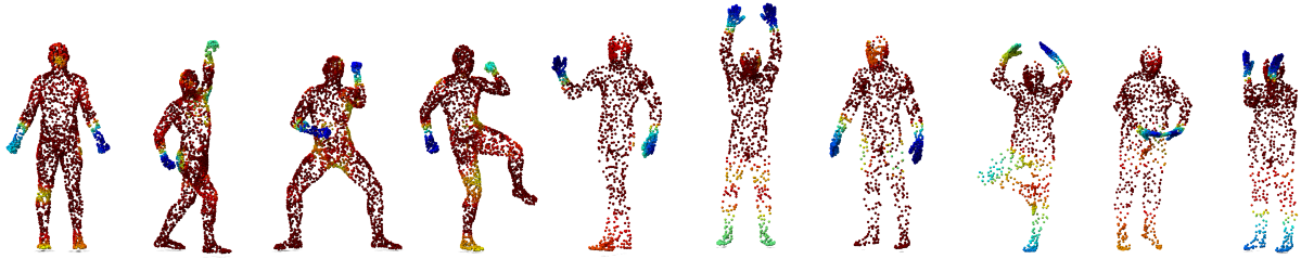
Figure 5: Distance map in the descriptor space computed using LSCNN on point clouds. A point on the reference shape (leftmost) is compared to all other points on the same and on other shapes (four from SCAPE and four from FAUST datasets). Small distances in the descriptor space correspond to cold colors.
