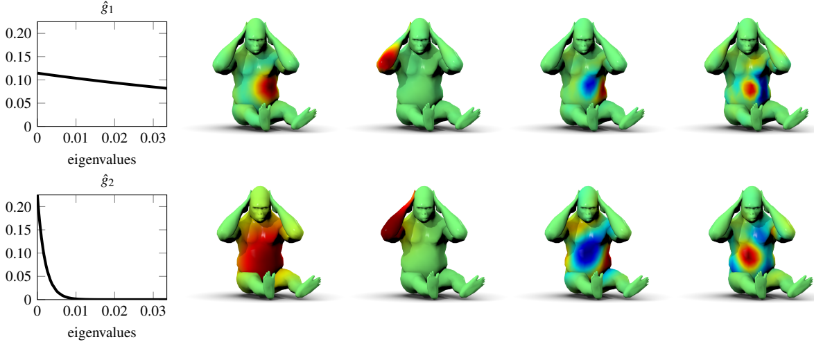
Figure 1: Examples of different WFT atoms g_{x,k} using different windows (top and bottom rows; window Fourier coefficients are shown on the left), shown in different localizations (second and third columns) and modulations (fourth and fifth columns).
